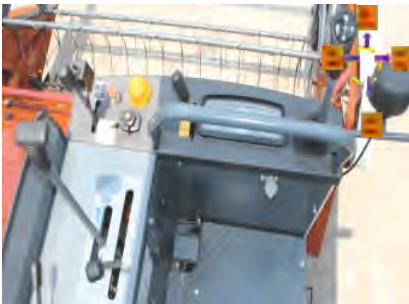
Single maneuvering lever makes machine easy to operate
