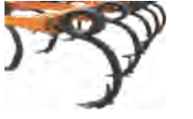
Double coil tyne of EN-45 material
