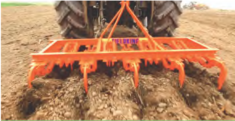
Spring having more capacity of absorbing shock
