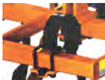
Double coil spring action tyne
