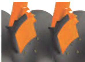
Boron steel disc with scraper attachment
