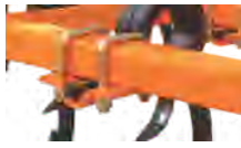
U clamp for attachment & adjustment of tyne
