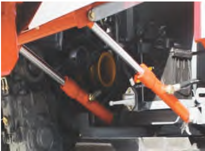
Double oil cylinder header assembly for better stability
