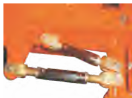
Turn buckle for adjusting of the plough
