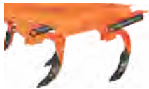
Shovel is made of EN-42 material
