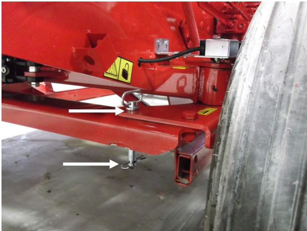
Figure 7 — Locking the Steering Before Towing
