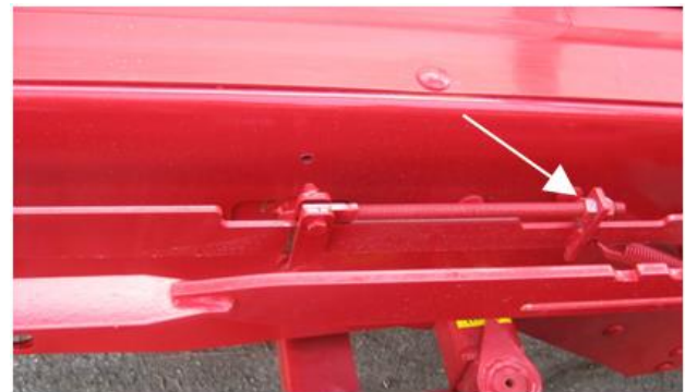
Figure 45 — Adjusting the Pusher Trigger (nuts)
