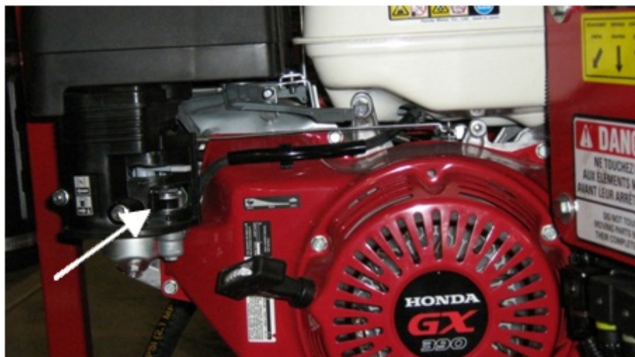
Figure 4 – Closing the fuel valve
