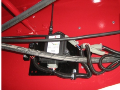
Figure 7 – The receiver of the remote steering
