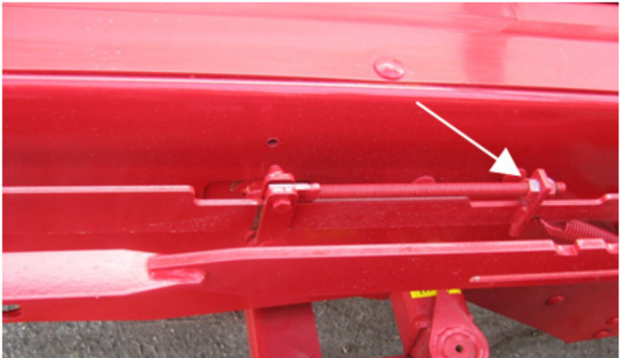
Figure 47 – Adjusting the pusher trigger (nuts)
