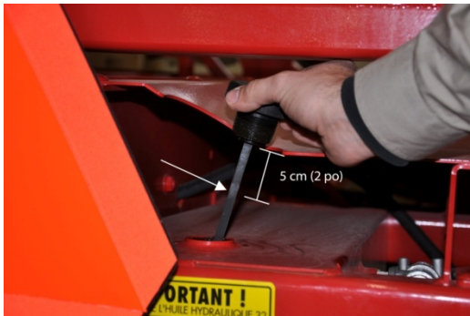
Figure 5 – Oil in Hydraulic oil tank
