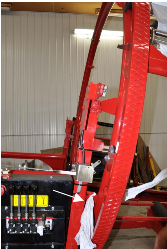
Figure 18 – Attaching the plastic film
